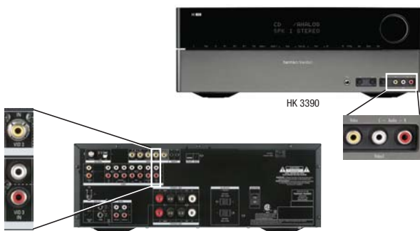
Figure 17 – Front- and Rear-Panel Video 3 A/V Inputs
